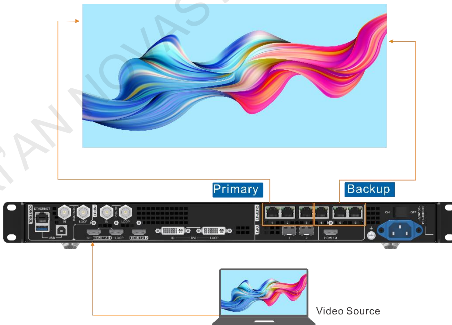
Figure 5-27 Ethernet port backup connection
