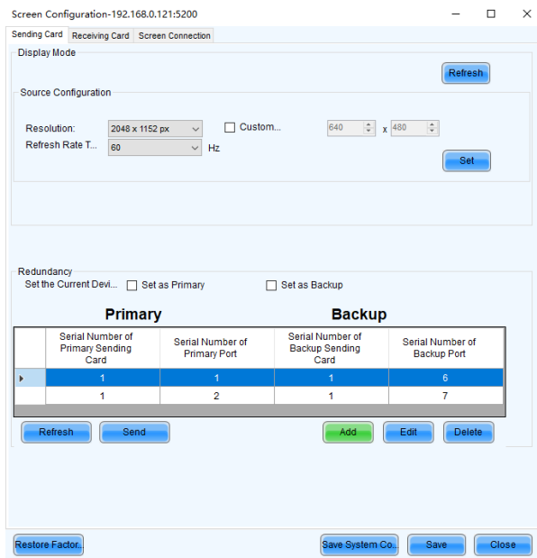
Figure 5-30 Primary Ethernet ports
