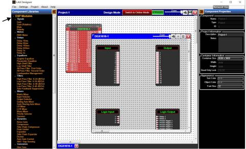
Processor Module – DSP Schematic Design Page
