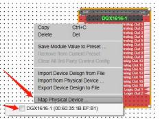
(This Mapping procedure can be done later if you have no physical processor to connect to at this time. Simply continue with your DSP design work, save as you go, and Map the software processor to the physical processor when one is connected and when you want to be able to transfer/save your DSP design work into the physical processor device)
