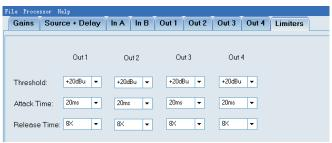
Output power limiter, including Theshoid, Attack Time, Release Time setting to control out1, out2, out3, out4.
