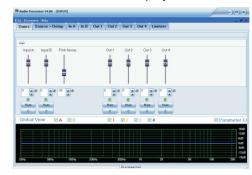
**Sub-menu:** Gains, Source+Delay, InA, InB, Out 1, Out 2, Out 3, Out 4, Limiters select then access: Gain Control, Source+Delay, Input channel 1, Input channel 2, Output channel 1, Output channel 2, Output channel 3, Output channel 4, Output limits. Each sub-menu can set relevant parameters.
